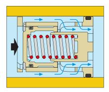
In this case, the regulating piston remains in equilibrium without compressing the spring and gives the medium the maximum free flow area. In practice, the piston acts as a fixed regulator and thus the flow through the AUTOFLOW® depends solely on the differential pressure.
