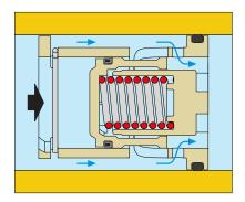
In this case, the piston compresses the spring fully and only leaves the fixed geometry aperture for the medium to pass through.
