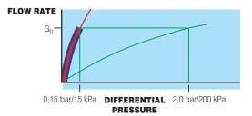
$Kv_{0.01} = 0.258 \cdot G_0$  Range  $\Delta p \ 15 \div 200 \text{ kPa}$  where  $G_0 = \text{nominal flow rate}$
