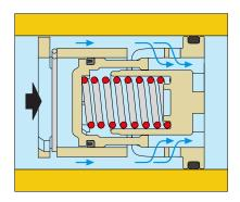
If the differential pressure is contained within the control range, the piston compresses the spring and gives the medium a free flow area to permit regular flow at the nominal rate for which the AUTOFLOW® is set up.
